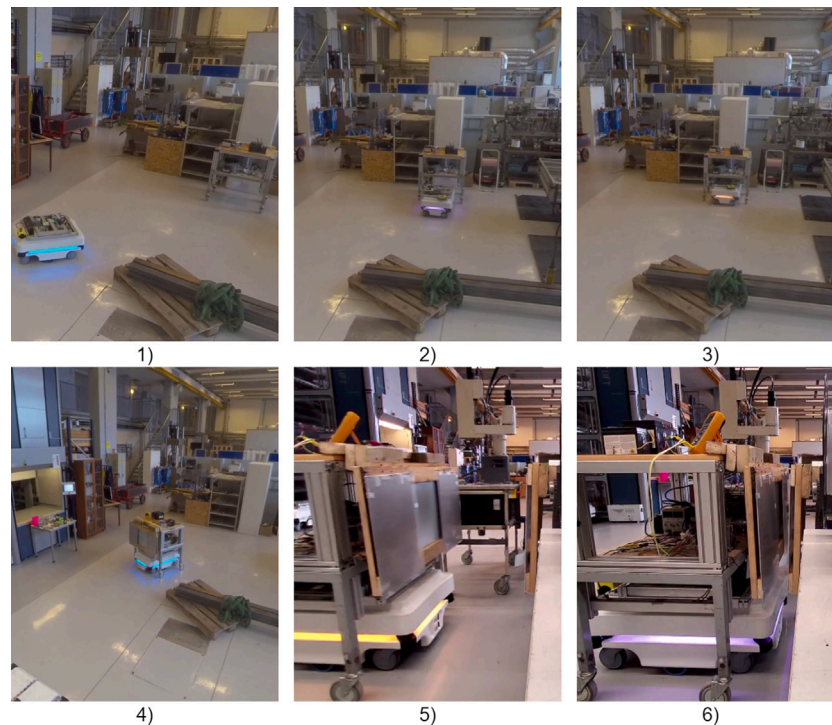
Fig. 12. Demonstration of how the CPT is implemented into the RMS: The mobile robot drives to pick up a full battery platform (step 1 to 4) and transports it to the charging RMS (step 5 to 6).
