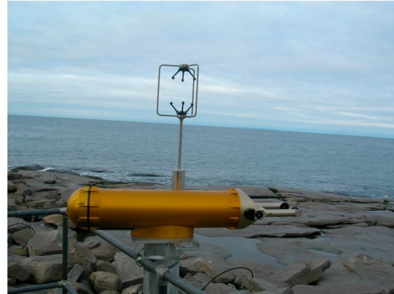
FIG. 2. The DMT CIP and the Gill sonic anemometer/thermometer mounted on the foghorn platform on Mount Desert Rock.
