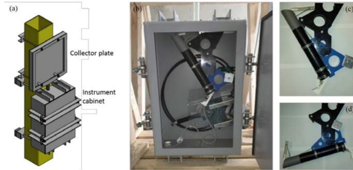
Figure 3. (a) Technical drawing of the collector plate and instrument cabinet assembly mounted on a vertical column, (b) Internal view of the instrument cabinet, (c) Close-up of tipping bucket in upright position, (d) Close-up of tipping bucket in tilted position.
