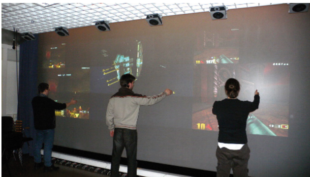
Figure 1: Two persons playing Q3A and one person playing Homeworld simultaneously on a 7x4 tile display wall. Q3A runs on 2x2 tiles to the left and right, and Homeworld on 3x3 tiles in the middle.
