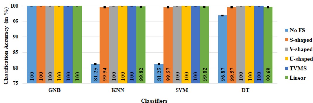
Fig. 6. Performance (average classification accuracy ± SD) of different BPSO setups for CKD prediction. Here, the term “No FS” indicates the performance of an individual classifier without using the BPSO-based feature selection.
