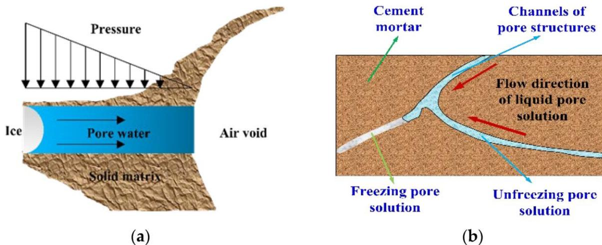
Figure 5 hydrostatic pressure and osmotic pressure model. (a) Hydrostatic pressure principle ; (b) Osmotic pressure principle, Guo et al. (2022)
