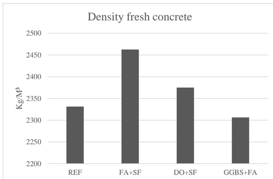
Figure 8 Density of fresh concrete in this trial
