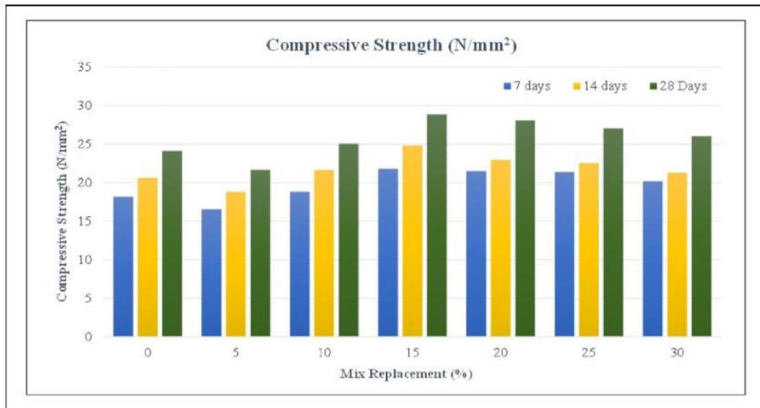
Figure 1 Compression strength of mixtures containing various amounts of dolomite, Gusain (2022)
