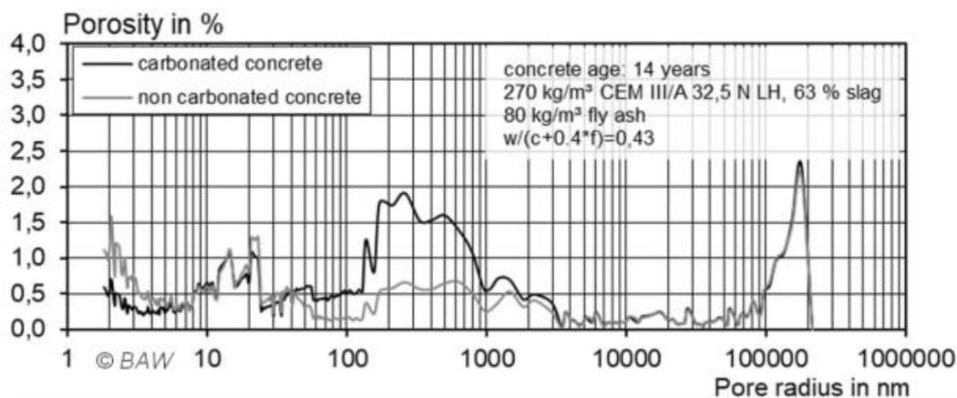
Figure 14 Changes in pore distribution on carbonated concrete samples, Hasholt et al. (2022)
