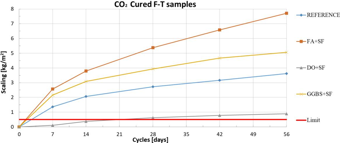
Figure 10 F-T results for CO<sub>2</sub> cured samples
