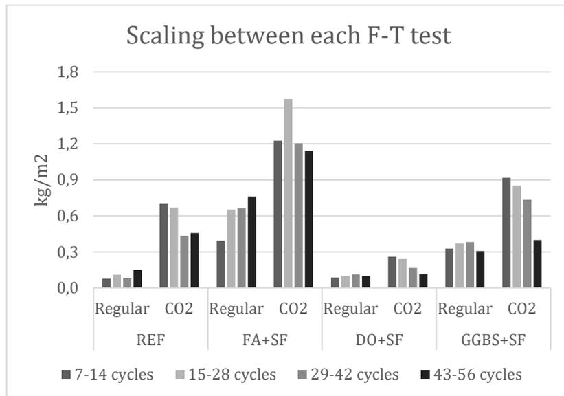
Figure 15 Scaling between F-T test days
