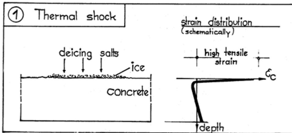
Figure 6 Thermal shock to a concrete surface layer, caused by application of a de-icer to a frozen surface covered by ice, Rønning (2001)
