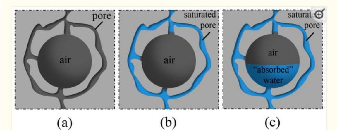
Figure 3 Schematic depicting capillarity and absorption of water by air diffusion: (a) Before immersion in water; (b) After immersion in water; (c) During F-T, Luo (2022)
