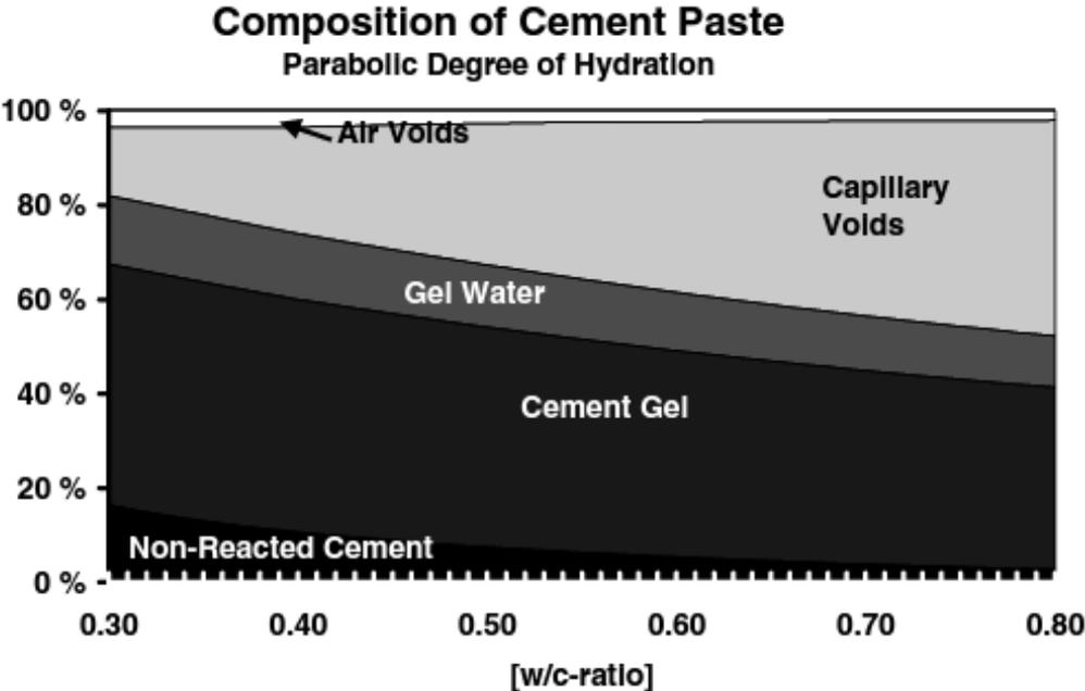
Figure 2 The effect of w/b-ratio on pores, Rønning (2001)
