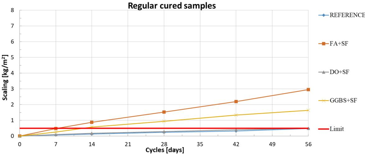
Figure 9 F-T results for regular cured samples
