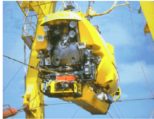
Fig. 2 - The Nautilé is a manned submarine designed for observing and operating at depths reaching 6000 metres. The submersible capable of exploring 97% of the world's ocean floors (IFREMER).
