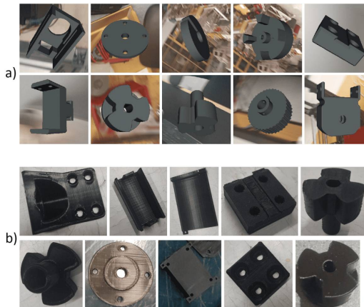
Fig. 2. The cycle GAN training approach: a) is the generated images, where backgrounds have been inserted, and b) is the real 3D printed parts used to train the cycle GAN.
