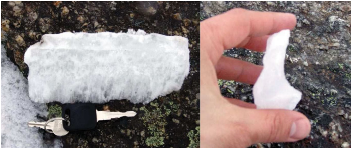
Figure 4: Glaze ice from a wind turbine blade [14]
