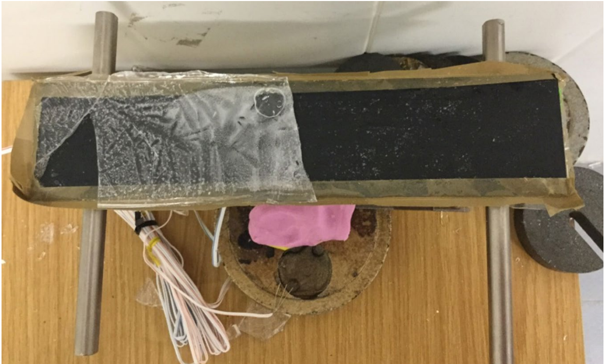
Figure 24: Failure in a 5 mm ice sample
