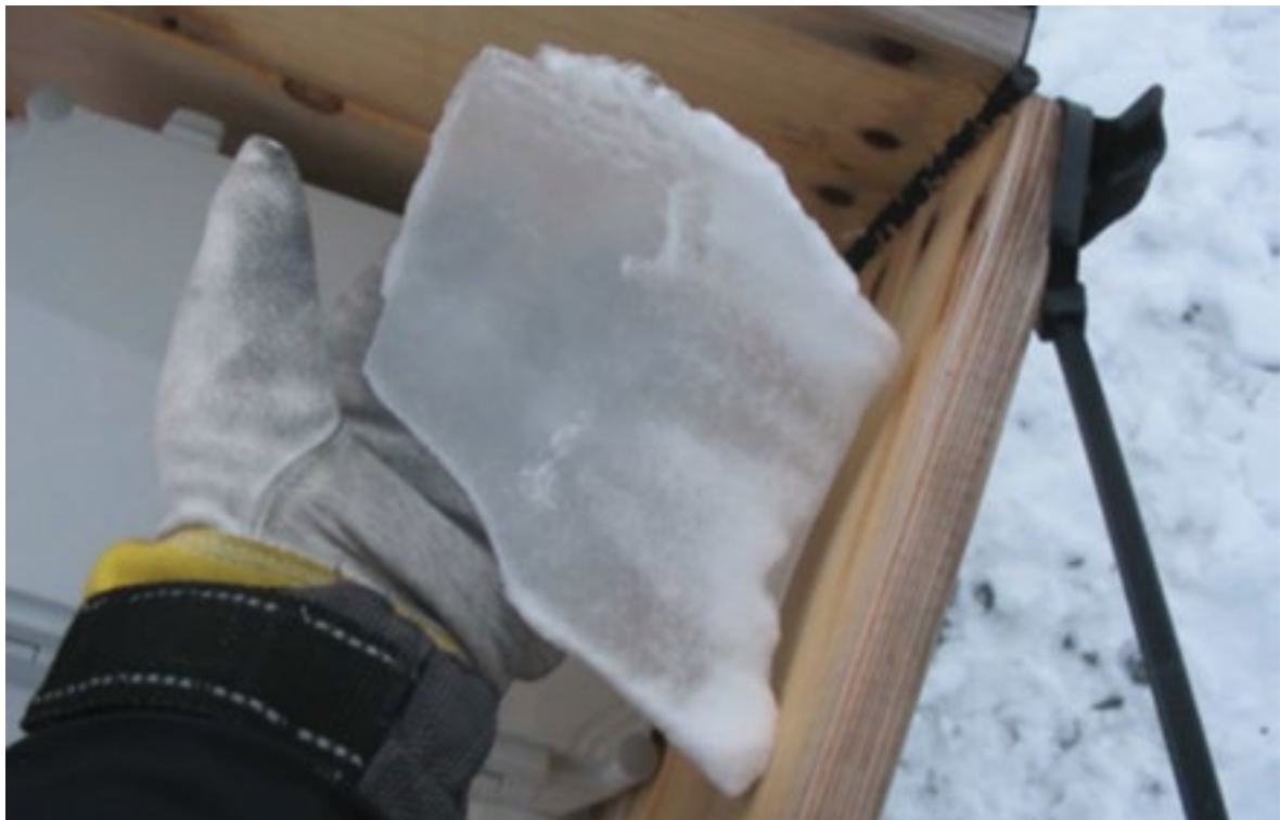
Figure 1: Piece of ice shed from a turbine in Nygårdsfjell wind park, Norway [12]
