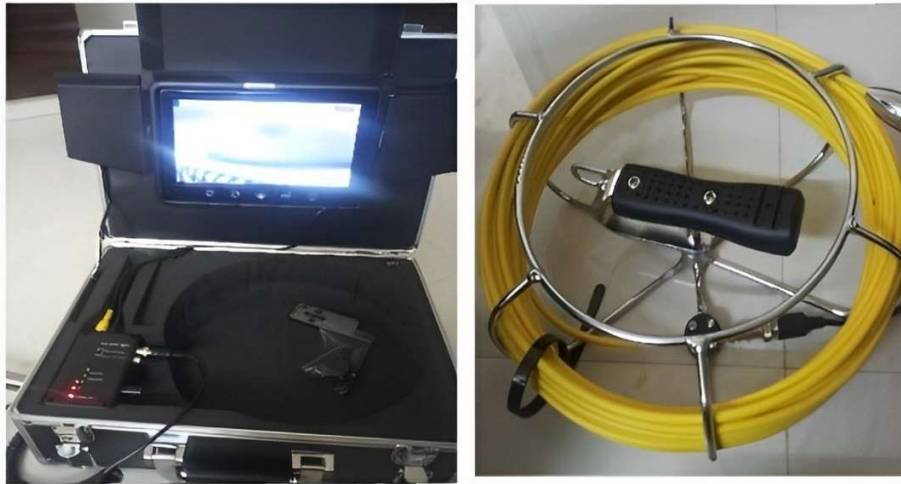
Figure 18 Watertight sewer camera employed for frame capture
