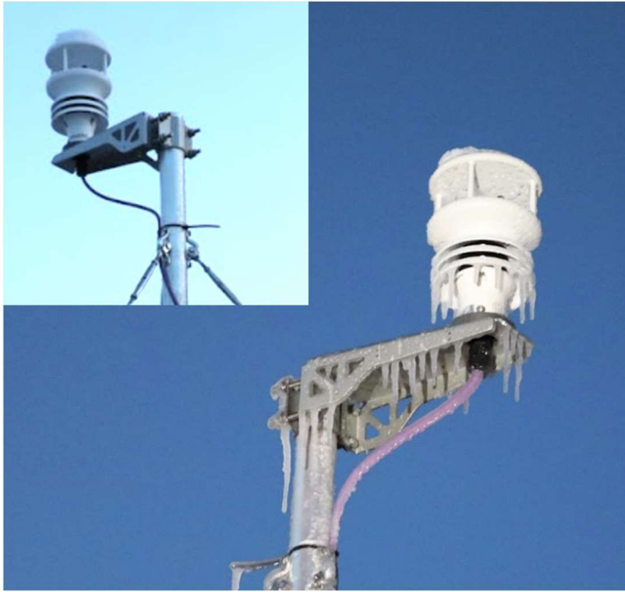
Fig. 14 Weather station mounted on the steering tower before (left) and after (right) the deicing procedure.
