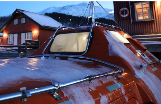
Fig. 12 Steering tower with the windows and the air inlet (on the right) after deicing.
