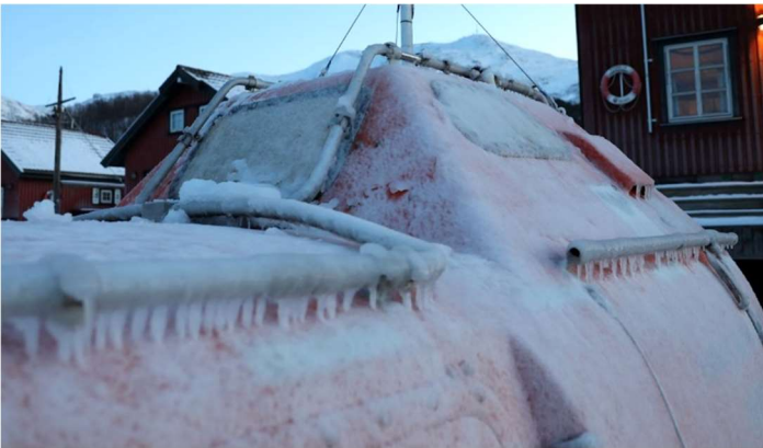
Fig. 11 Steering tower with the windows and the air inlet (on the right) before deicing.
