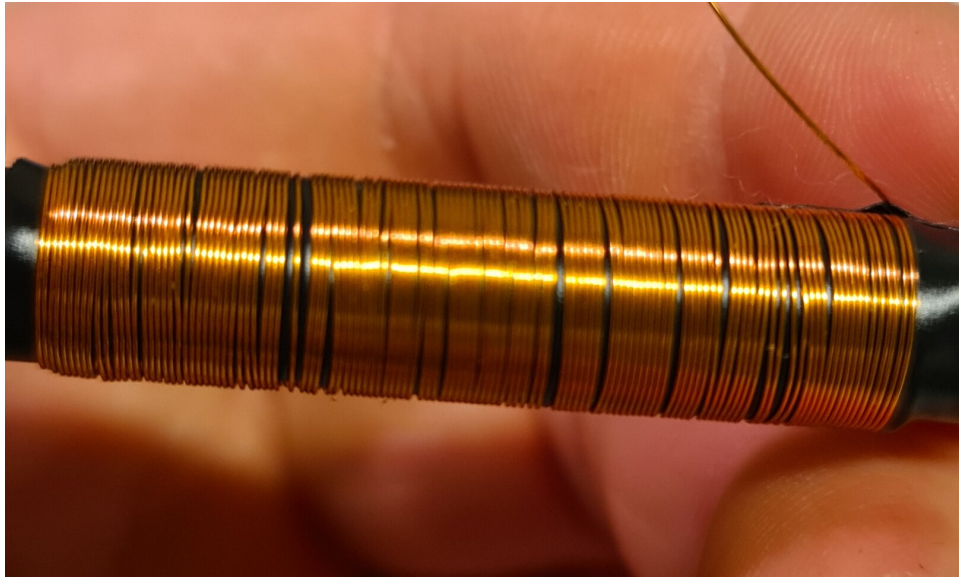
Figure 5.14: The 300-turn antenna utilized to investigate whether increasing the number of turns can enhance the antenna's receptive range.
