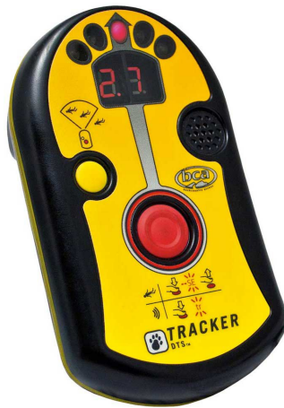
(c) BCA tracker, the first "digital" beacon, came out in 1997. This beacon featured two antennas running at 457 kHz and could indicate the direction and distance of the buried victim.
