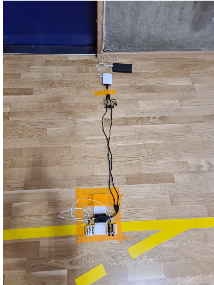
Figure 6.7: To test the effect the Raspberry Pi had on radio interference, tests were done with the Raspberry Pi as far away as the USB cables would allow.
