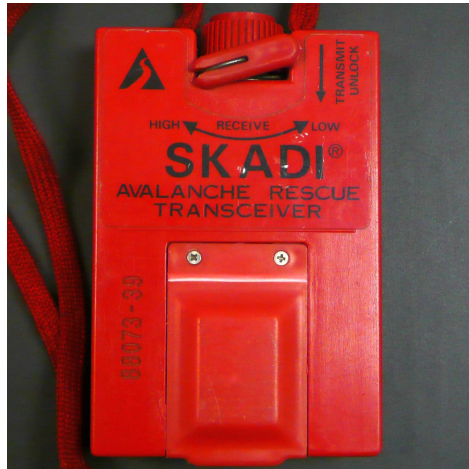
(a) The SKADI avalanche transceiver, one antenna broadcasting a signal at 2.275 kHz. This was the first commercial avalanche beacon, which started retailing in 1970.
