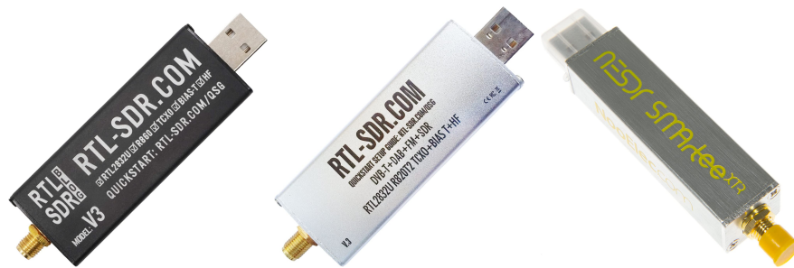
Figure 3.5: This is a small assortment of various RTL-SDRs. Despite their distinct appearances, they all employ the same chipset internally.
