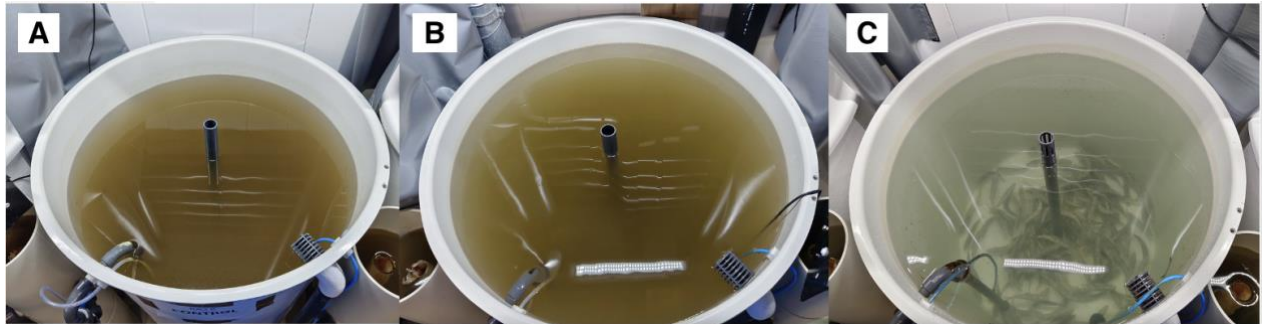
Figure 23: Fish tanks with different treatments on the last day of the trial. A) is the control treatment, B) is PAA treatment and C) is ozone treatment. Control and PAA treatments tanks are visibly more turbid than ozone treatment tank.
