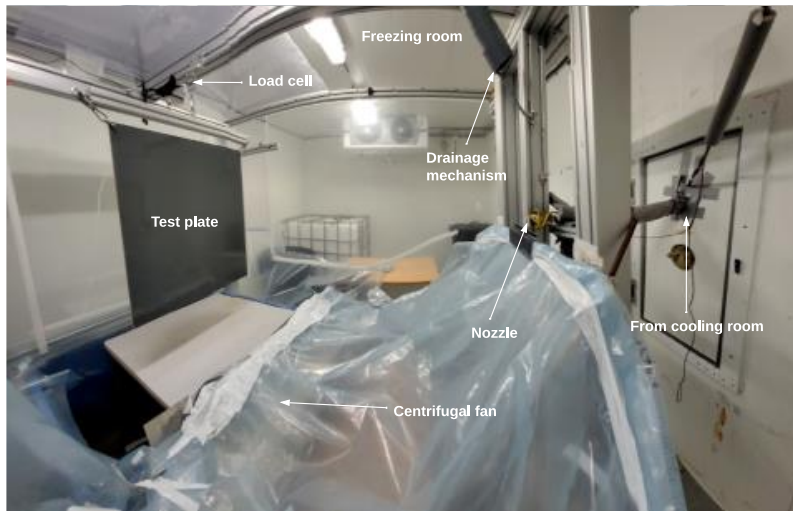
Figure 3: Freezing room setup
