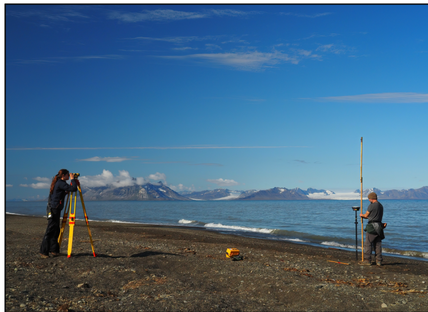
Figure 10: Mathilde and David conducting an optical sighting survey on the shoreline of Bogebecken to establish the elevation of the base of BKS1 in relation to the high tide mark on the 26th of July 2023. Optical sighting scope on the left, operated by Mathilde and measuring pole on the right, held by David. Photo: Mark Furze.
