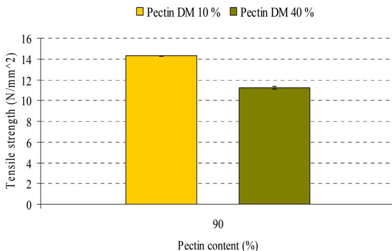
**Figure 29: Tensile strength of mini – tablets containing pure pectin type (DM10% and DM 40%) (n= 5)**
