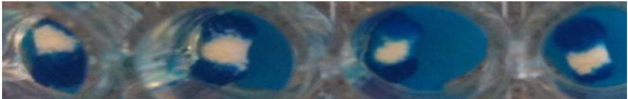
**Figure 32:** Results of simulated wetting time for mini-tablets in pH 6.8 solution A) 90 % pectin 10 % B) 90 pectin 40 % (n=5)
