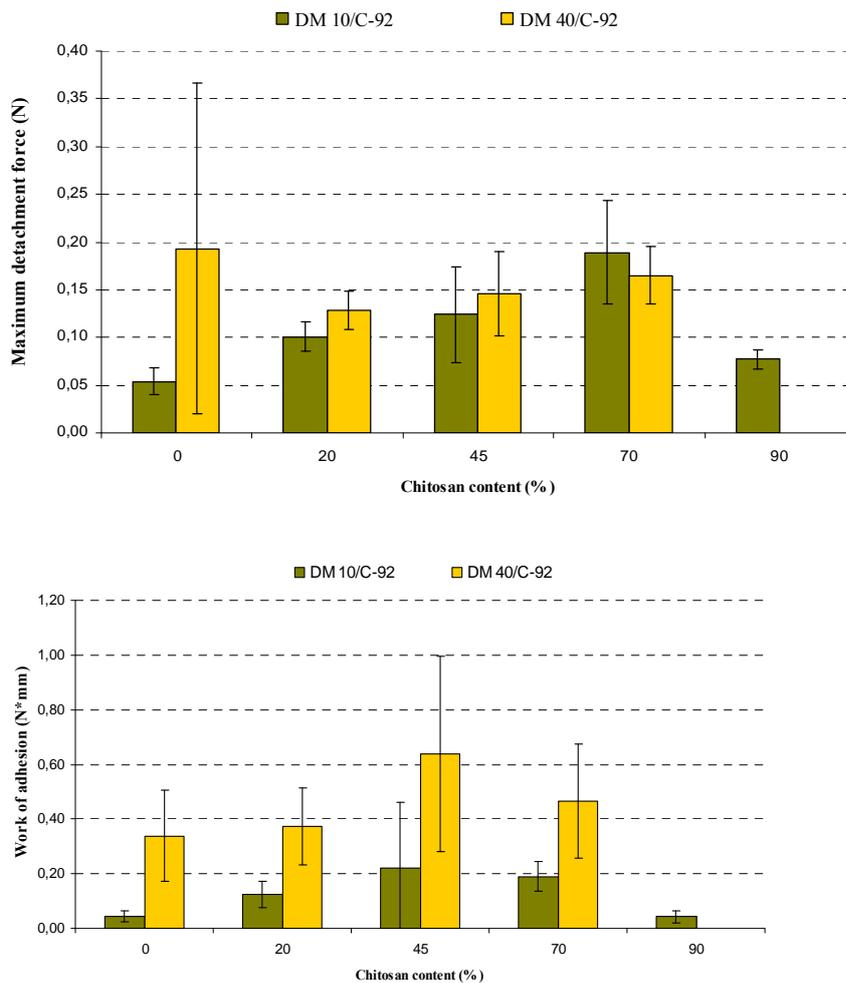
**Figure 22:** Mucoadhesion of 11 mm tablets to cow vaginal tissue for various combinations of chitosan:pectin ratio A) Maximum detachment force B) Work of adhesion. Data presented as mean  $\pm$  SD (n=3). (n=10)
