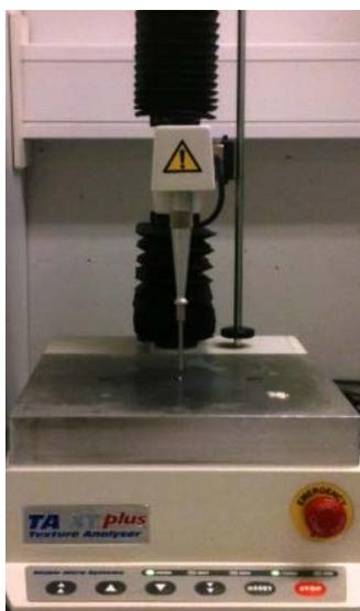
**Figure 8:** Illustration of crushing strength measurement of mini-tablets by using Texture Analyser.
