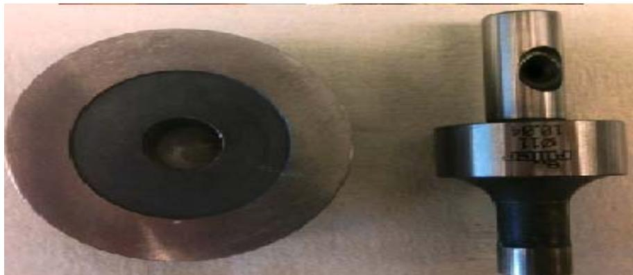
**Figure 6:** Tablet tooling A) 2 mm, concave multiple mini-tablet tooling. B) 11 mm flat-faced punch.
