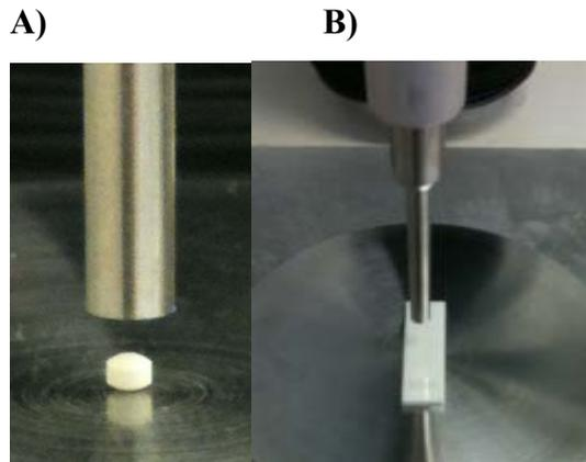
**Figure 9:** Illustration of A) measurement of height of a mini-tablet. B) Calibration for distance with calibration block.
