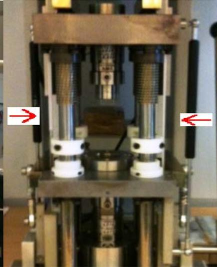
**Figure 5:** A) Schmidt ServoPress 450 A) Compression modul from IBR. Red arrows indicate the position of sensors which measures the distance
