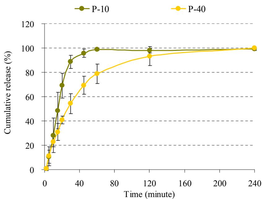
**Figure 19:** Drug release profile of metronidazole from mini-tablets containing 90 % pectin of various grade (DM 10% and 40 %) A) in VFS pH 4.5 B) in VFS pH 6.8.;(n=3)
