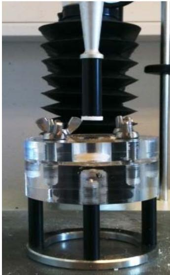
**Figure 12:** Picture of mucoadhesion rig and 11 mm tablet attached to the probe with a bilateral tape.
