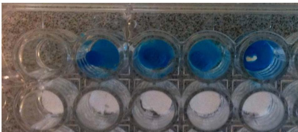
**Figure 15:** Photo of test set up: 96-titeplate with filter, sensient blue solution and mini-tablets. Fully coloured mini-tablets, confirming the end point of the test, can be seen in the back row,
