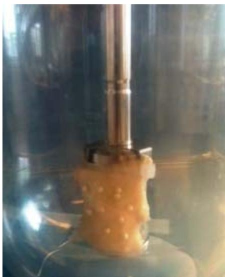
**Figure 14:** Experimental set-up of the rotating cylinder method showing how rectal tissue is fixed to the rotating cylinder and mini - tablets attached on the surface
