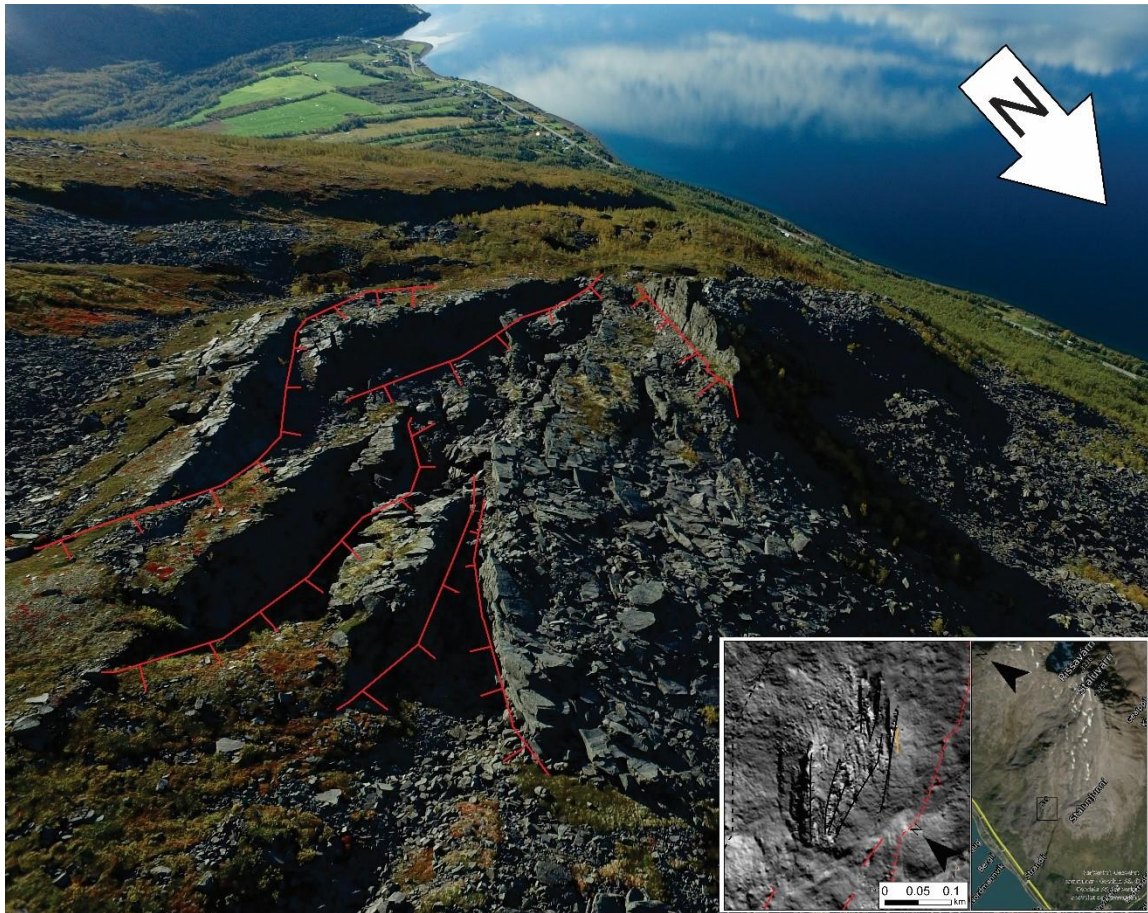
Figure 21: Large horst and graben system within the lower domain, which can be traced downslope towards the west as open fractures. Picture taken by Sindre Norheim 2018.
