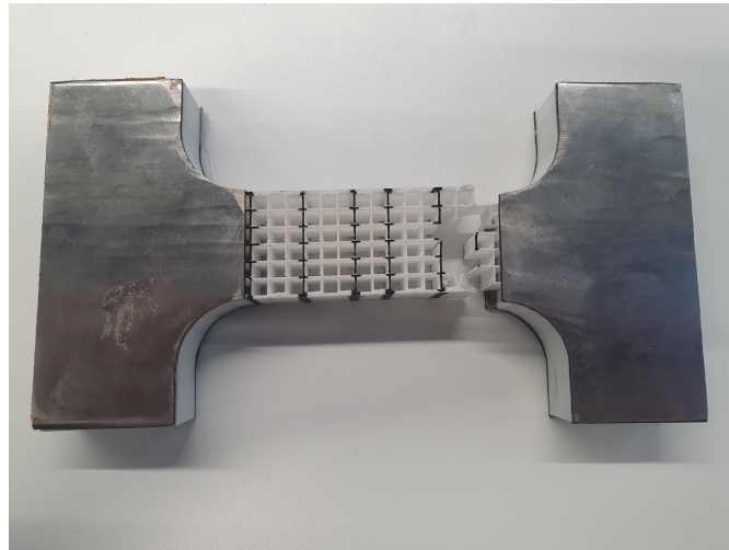
Figure 5.14: Fracture of dog-bone specimen number 3, grid pattern, raster angle 0^\circ , and 20% infill.
