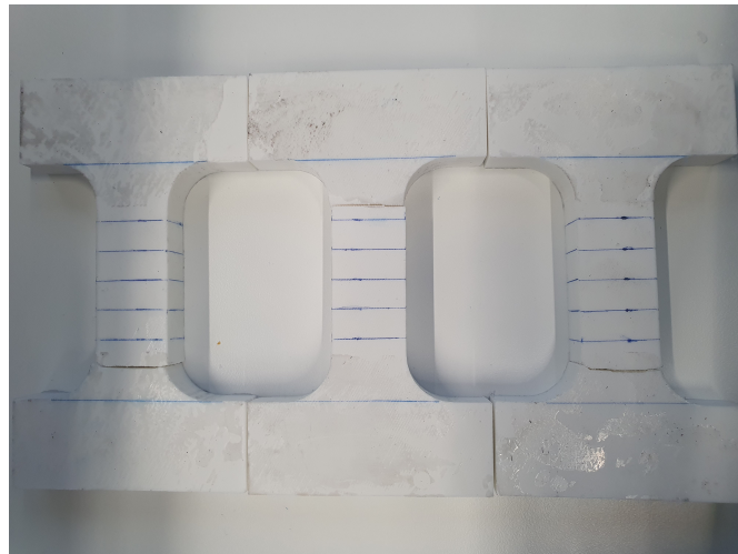
Figure 5.12: Dog-bones after tensile test for line pattern with CLT raster angles.
