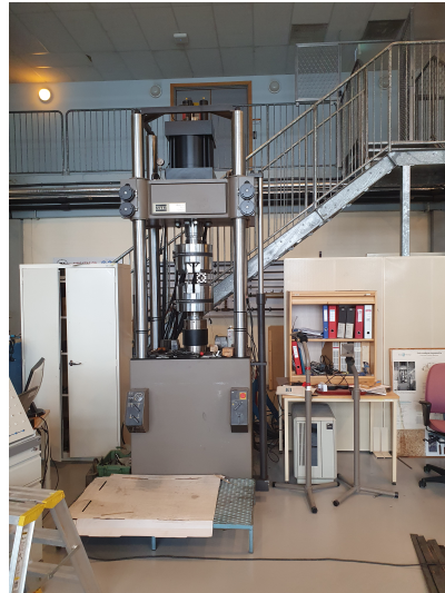
Figure 2.3: Material test machine used to perform material test.
