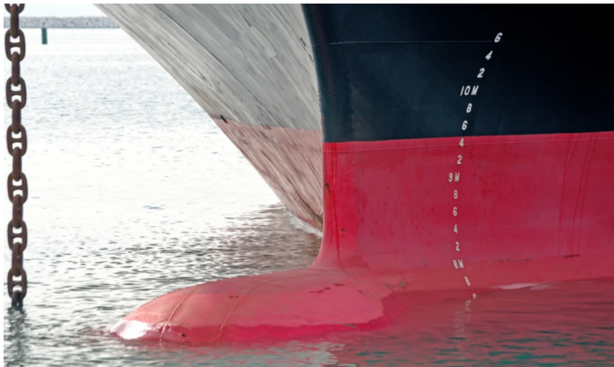
Figure 2: Draft scale painted on a ship [4]
