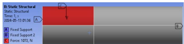
Figure 53: Loading and boundary conditions for side roller cylinder[26]
