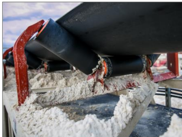
Figure 2–3 Superior Industries Moxie rollers [15].
