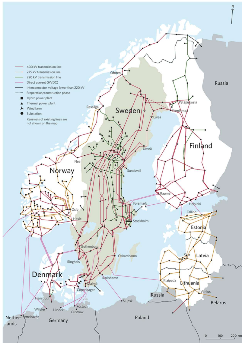
Figure 3.2 - Transmission lines in the Nordic countries, from (Svenska Kraftnät, 2023, September 29)
