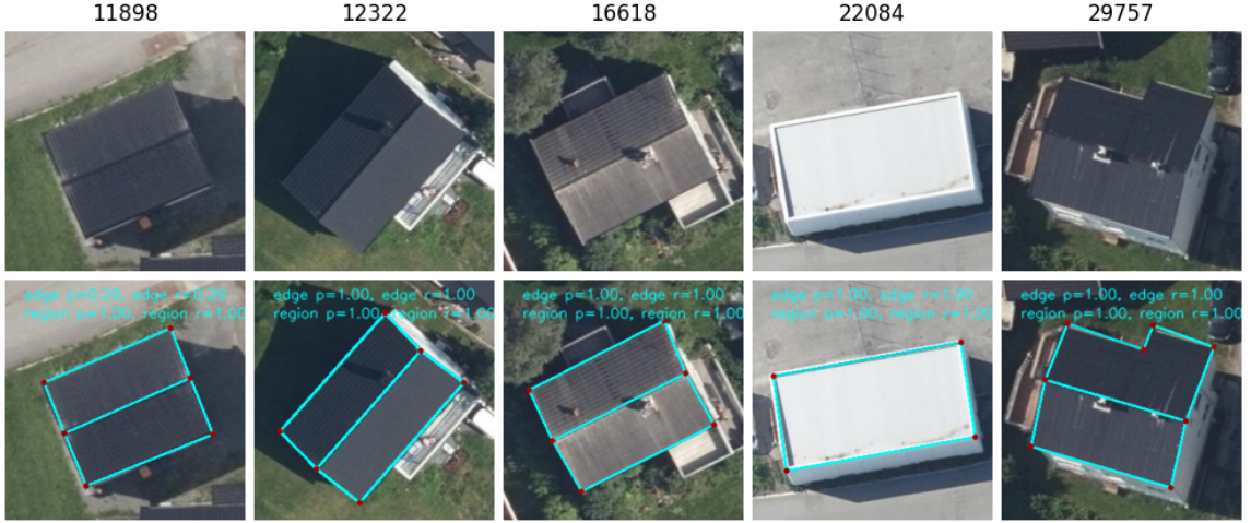
Figure 18: Five buildings used in the 3D reconstruction with HEAT structure inferences. The images of the five remaining houses can be found in Appendix 8, Figure 29. Upper panels: Source images. Bottom panels: Inferred graphs. precision and recall for edge and region prediction is shown.
