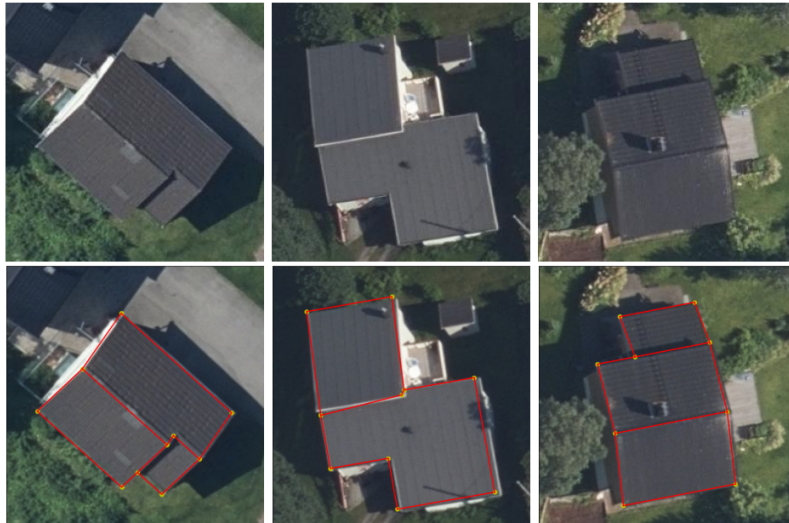
Figure 28: Examples of buildings with multi-tiered roof structures. The graphs in the second row are transformed SFKB graphs.
