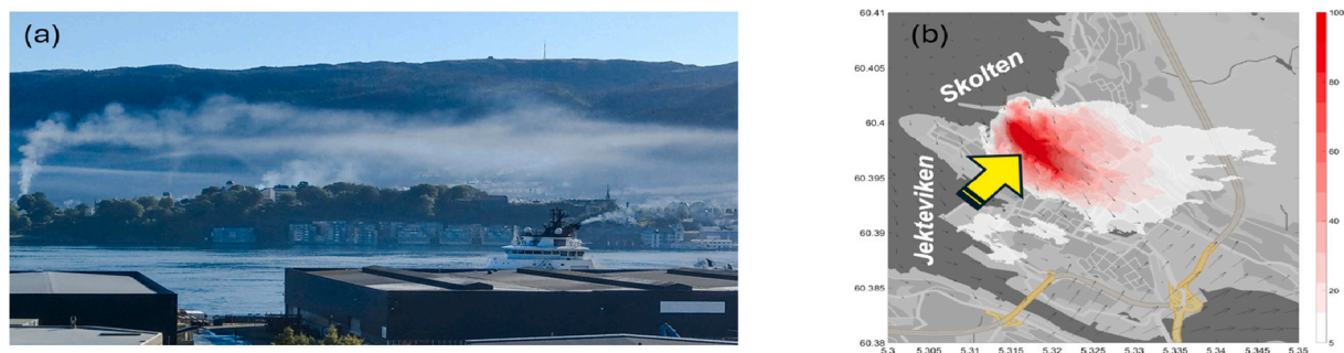
Fig. 6. (a) A visual example of air pollution in the port of Bergen (“Bergens Tidende” newspaper, 23 July 2018). (b) PALM simulations of this air pollution episode (model resolution 15 m, the simulation domain included the whole Bergen municipality). NO x concentrations are shown by red color shades, wind speed and direction by black arrows. The yellow arrow shows the standpoint and direction of the image in (a). (For interpretation of the references to color in this figure legend, the reader is referred to the web version of this article.)
