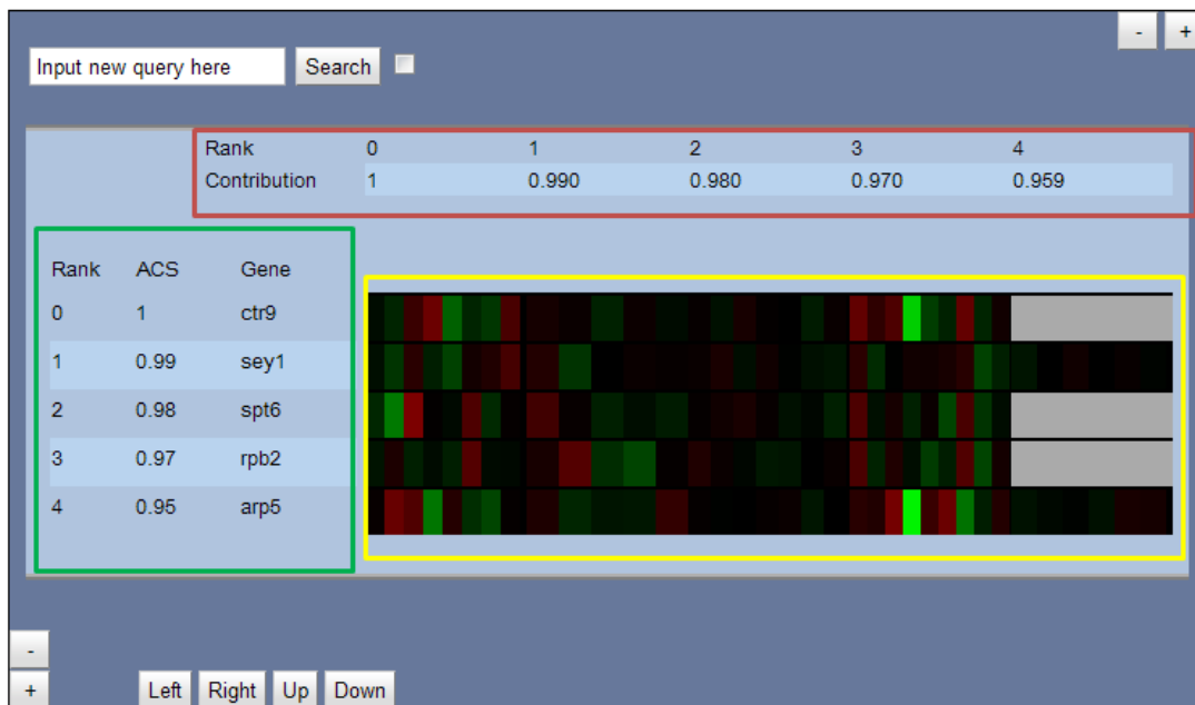
FIGURE 18 - THE THREE VIEWS THAT REQUIRE DATA IN THE HEAT MAP WIDGET. THE RED ZONE IS THE HORIZONTAL HEADER, THE GREEN ZONE IS THE VERTICAL HEADER AND THE YELLOW ZONE IS THE HEAT MAP CONTAINER.
