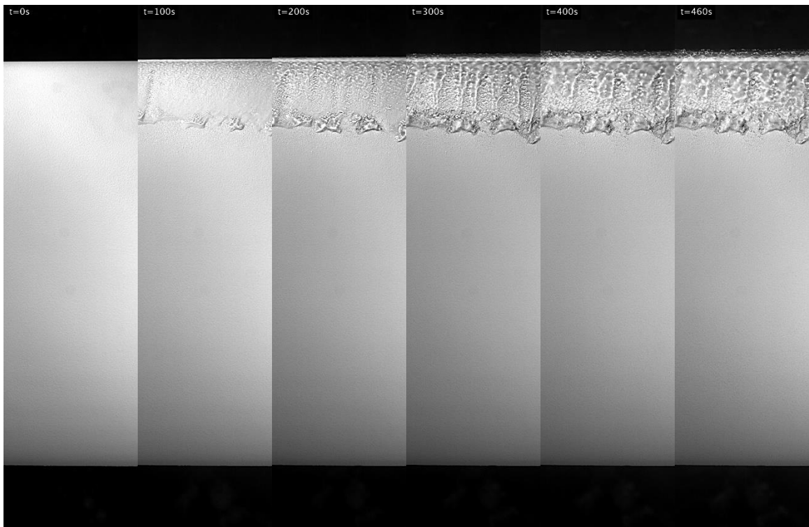
Fig. 3: Ice accretion on the surface of clean UAV wing at glaze ice condition (0,100,200,300,400,460 seconds).
