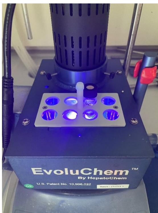
Figure S3. Photoreactor setup. The photoreactor was placed onto a stirring plate, topped with the light source of choice, and filled with a thermostatic mixture (glycerol/H 2 O 2:1) kept at set temperature by recirculating through the cooling/heating bath unit (not visible on figure). Reaction vials were immersed in the thermostatic fluid and held in place by the holder, which allowed an even light irradiation of all reaction mixtures.
