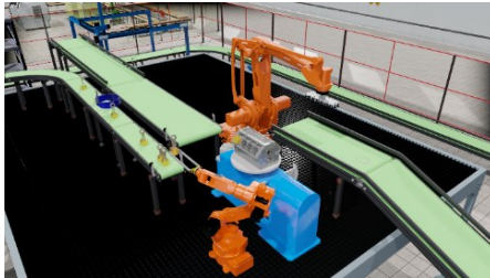
Fig. 2 Assembly of engine and piston
