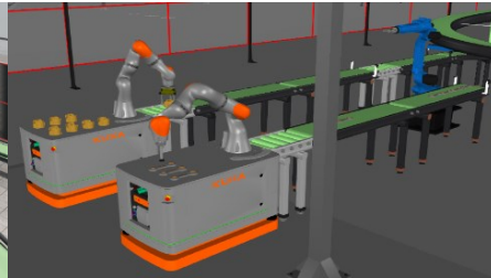
Fig. 3 AGV transportation of piston components
