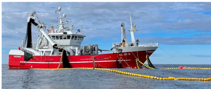
Fig. 4. A typical medium sized, coastal Norwegian purse seine vessel. The vessel shown (MS Vestbris) was used in sea trials to investigate Atlantic bluefin tuna live storage feasibility. MS Sjøarmør II (the other vessel used in the trials) was similarly designed.
