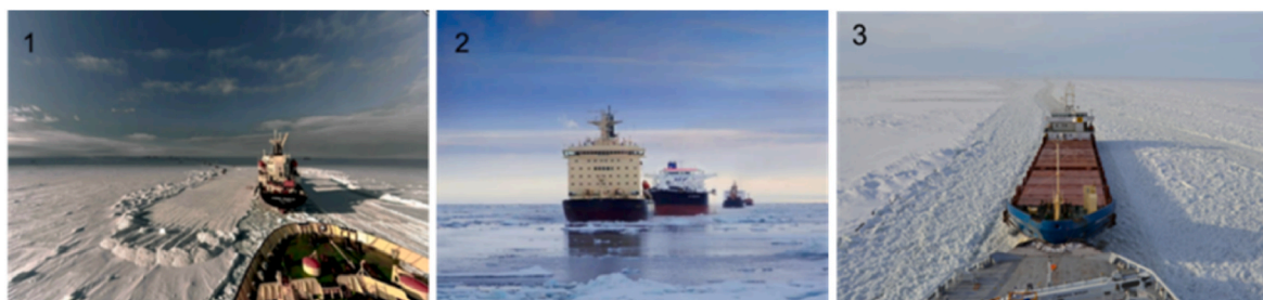
Fig. 1. Navigation modes under icebreaker assistance: 1) Escort operation (PortNews, 2016); 2) Convoy operation (High North News, 2018); 3) Towing operation (Heinonen and Immonen, 2017).
