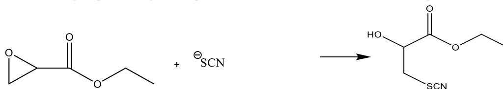
Scheme 8 Reaction scheme of epoxide ring opening with thiocyanate.
