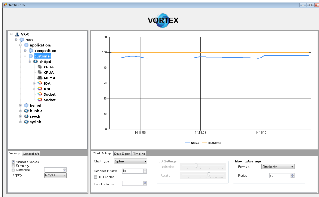
Figure 5.2: I/O utilization when operating with 10% of the available network resources, measured in Mbit/s.
