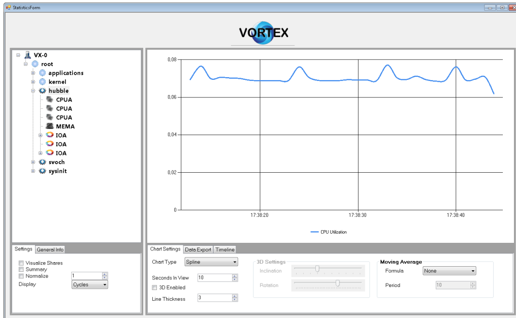
Figure 5.10: cpu utilization of the monitor at 10 requests pr second, measured in percent.
