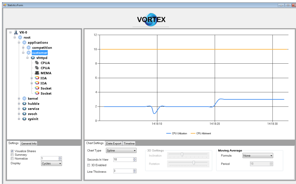
Figure 5.7: Cpu utilization after increasing the allotted network resources to 20%, measured in percent.
