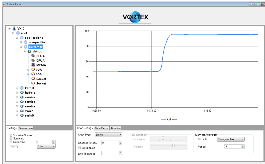
Figure 5.8: Application performance after increasing the allotted network resources to 20%, measured in requests per second.
