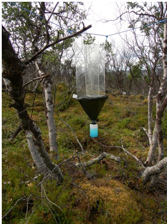
Fig. 3: Arrangement of a window crosstrap between two birch trees
