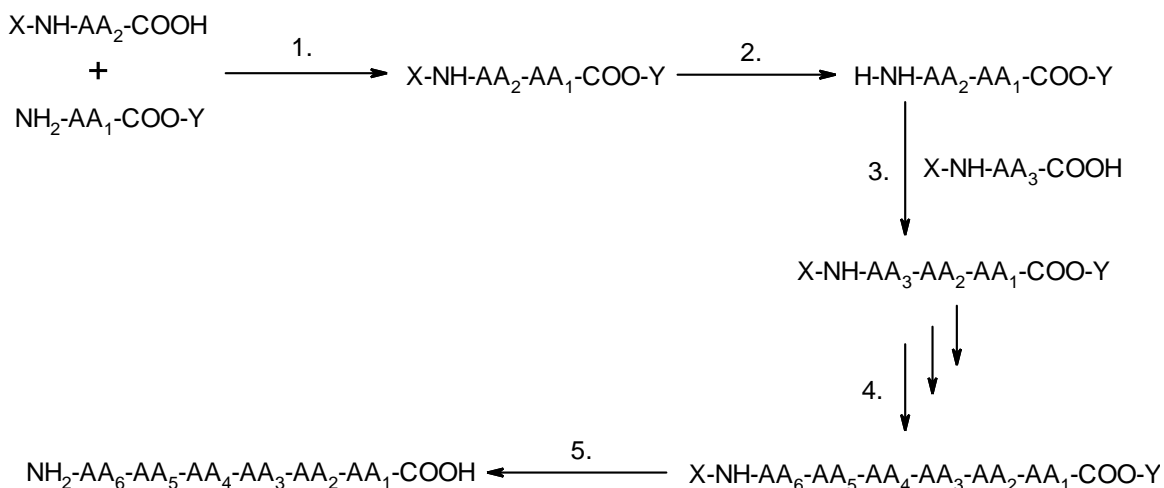
Scheme 3.10 The route of solution phase peptide synthesis.
