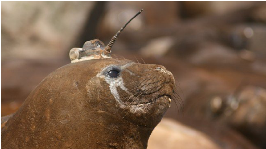
Figure 3.5: Sensor equipped Southern Ocean Elephant Seal ready to collect oceanographic data. Photo: Martin Biuw
