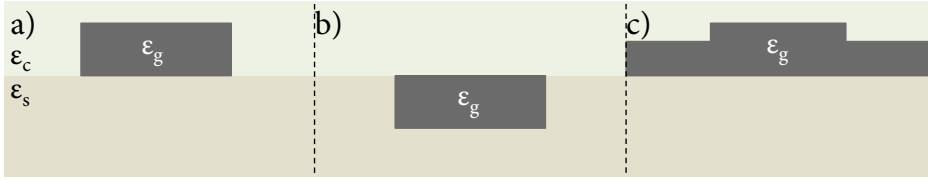
Figure 2.4: Rectangular a) strip, b) embedded strip and c) rib channel waveguides configurations.
