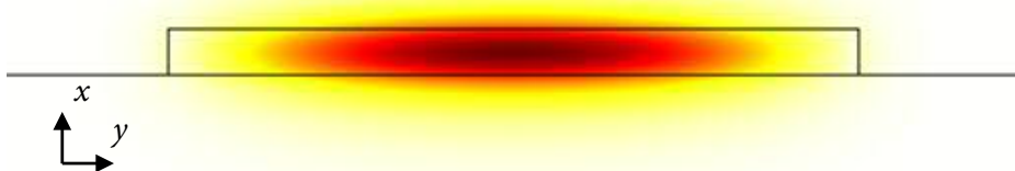
Figure 3.6: Plot of the field norm of the fundamental mode of a 3 \mu\text{m} wide and 200 nm high waveguide. Axis directions are indicated.
