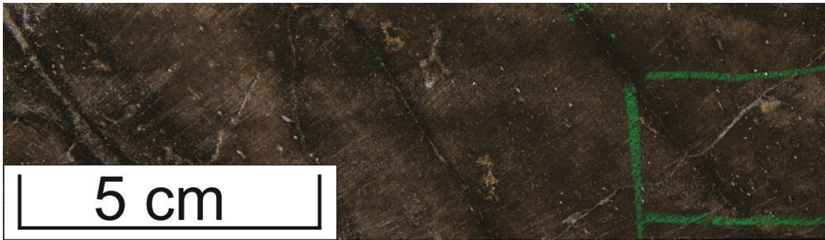
Figure 3.5: Core piece from 29.50 m to 29.65 m. The figure is from the part of the core which has the highest content of Au and As. This is clearly seen as numerous arsenopyrites (silver to whitish needles). The green square in the middle of the figure is the outline for the thin section.
