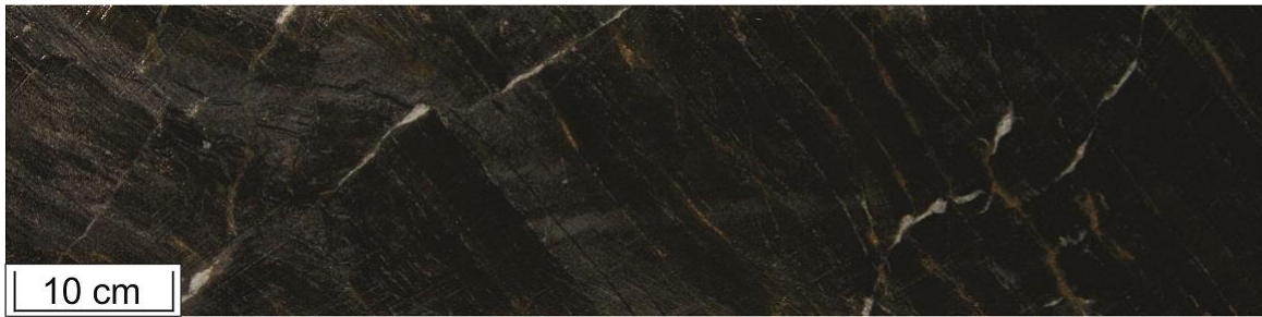
Figure 3.3: Core piece from 28.15 m to 28.80 m. the rock is dominated by fine grained quartz and micas and shows a laminated texture. The yellow/golden stripes are fine grained pyrite.
