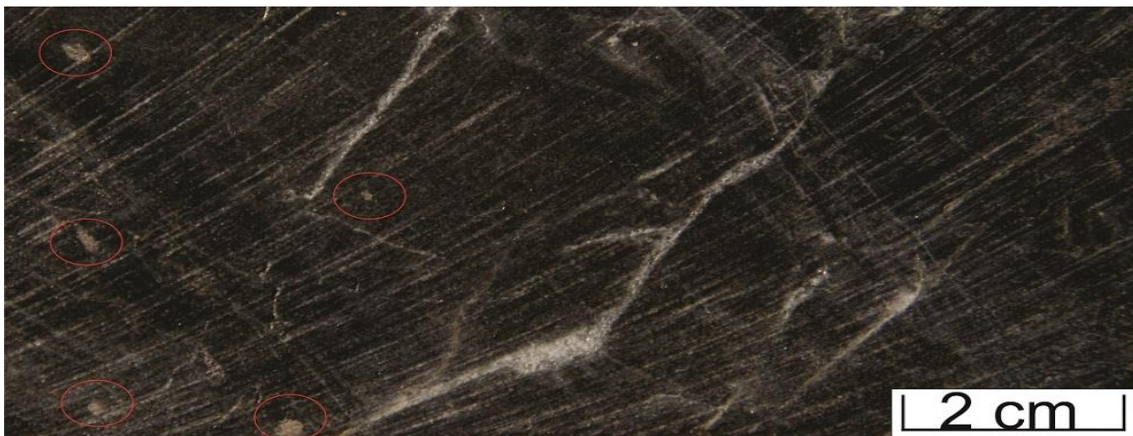
Figure 3.2: Core piece from 18.70 m to 18.80 m. The rock is dominated by fine grained quartz and micas with laminated texture. Pale red garnets are circled in red. Note the striation from the core saw going from the bottom left corner towards the upper right corner.
