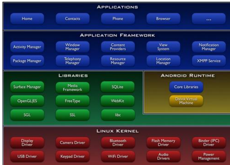
Figure 74. Android system architecture. Source 32
