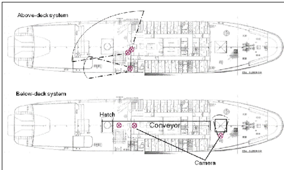
Figure 11. Final location and field of view for each of the cameras installed as part of the EM systems.
