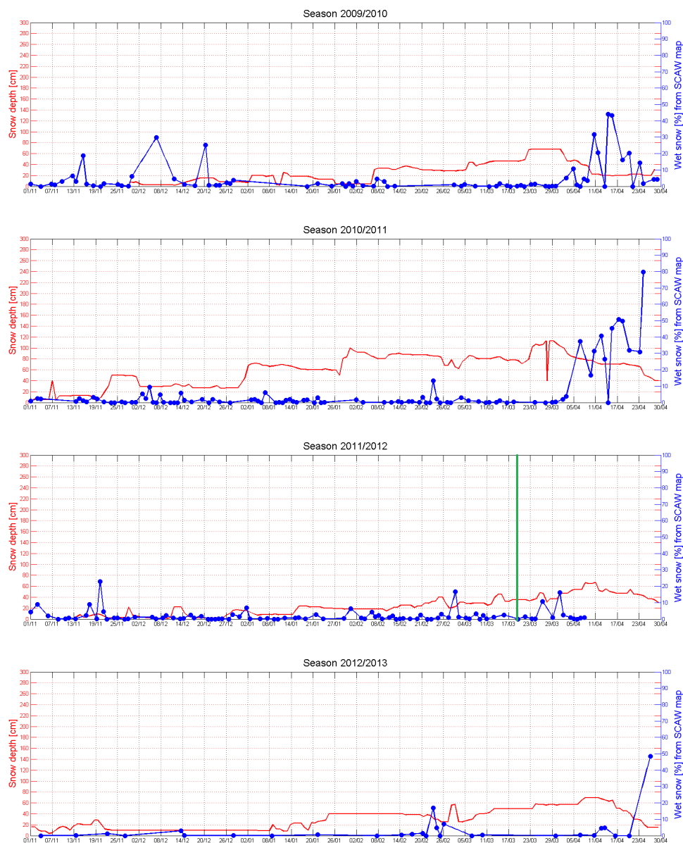
Figure 6.18: Detected wet snow fraction plot for avalanche site 4 for the winter seasons, starting with the 2009/2010 season in the top image, and ending with the 2012/2013 season in the bottom image. The green, vertical line in the second to last image marks the avalanche accident at Sorbmegaissa, 19th March 2012. Method 1 is used as reference method. The blue dots mark the real values for the SCAW wet snow fraction. The blue line shows the interpolated values of the wet snow fraction, and the red line shows snow depth.
