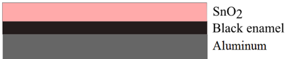
Figure 3.9: A schematic diagram of a Solar transmitting absorber.
