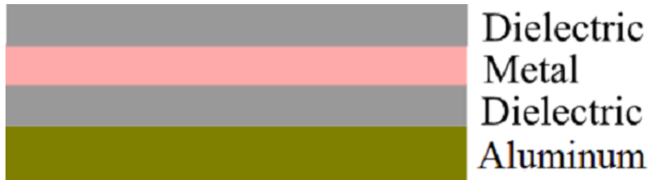
Figure 3.8: A schematic diagram of a multilayer solar absorber.
