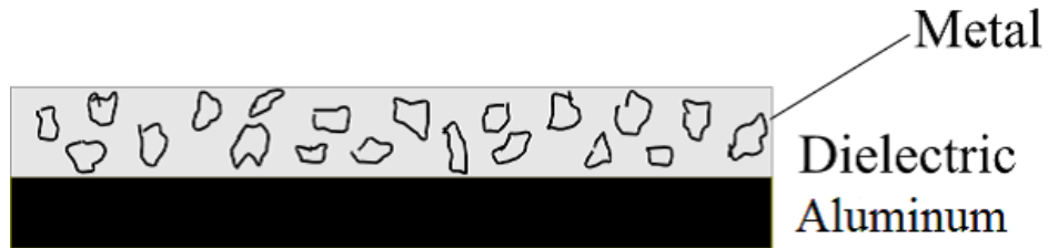
Figure 3.11: A schematic diagram of a Dielectric composite absorber.
