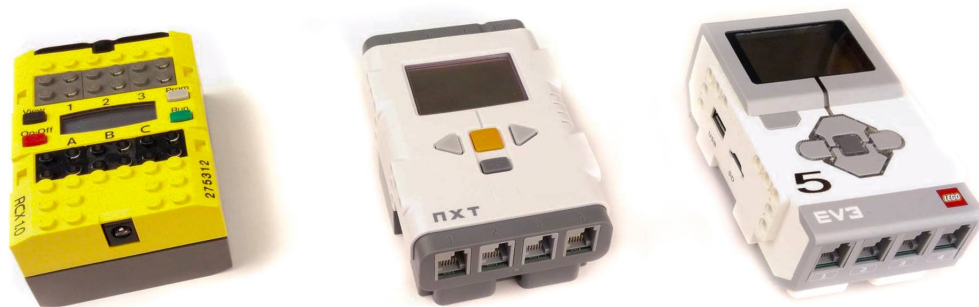
Figure 2.1: The programmable intelligent brick of each generation. Left RCX, Middle NXT, Right EV3
