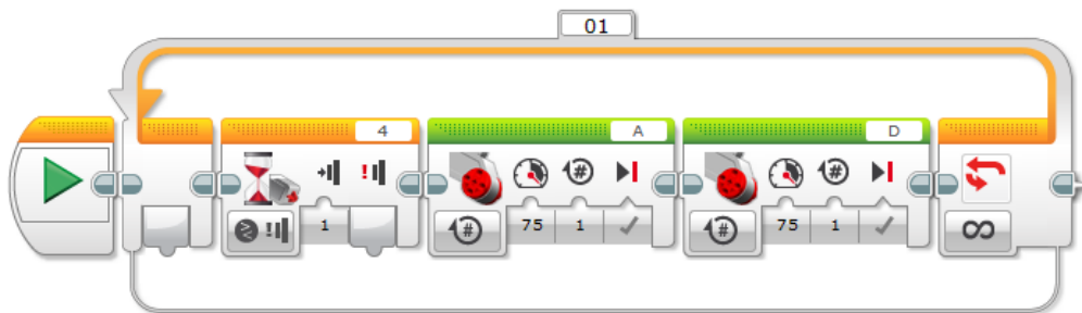
Figure 2.2: Shows a short program written in the default programming environment of the EV3. It is running an infinity loop around all the blocks. The first action inside the loop waits for the touch sensor on port 4 to be pressed. When pressed, the connected motor on port A rotates 360 degrees. Then the connected motor on port D rotates 360 degrees. Then the loop starts at the beginning again, waiting for the button to be pressed. This continues until the program exits.
