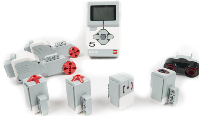
Figure 2.3: Main components in the EV3 education set, without the small motor
