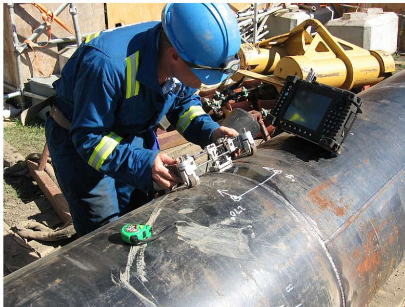
Figure 1.4: Ultrasound test of weld 2
