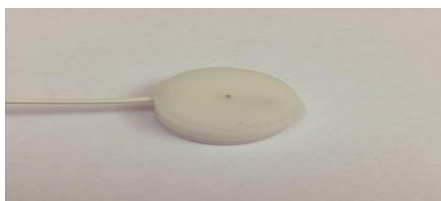
Picture 1. The electrode used to induce electric pulses (diameter 19mm, platina tip 0.2 mm)
