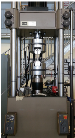
FIGURE 6: The MTS during tensile testing of a steel sample.
