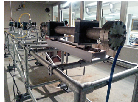
FIGURE 3: The shock tube. Driver section to the right (containing compressed air) and driven section to the left containing uncompressed water and a T-section for mounting the test specimen.
