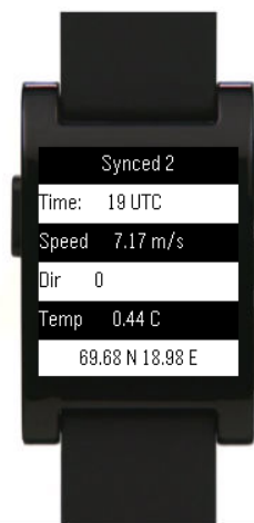
Figure 12.5 Example of point-forecasts on a Pebble smart watch. The actual location of the smart watch/cellphone is used for requesting the forecast.
