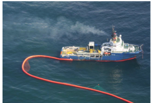
(b) Oil collected in the boom system.
