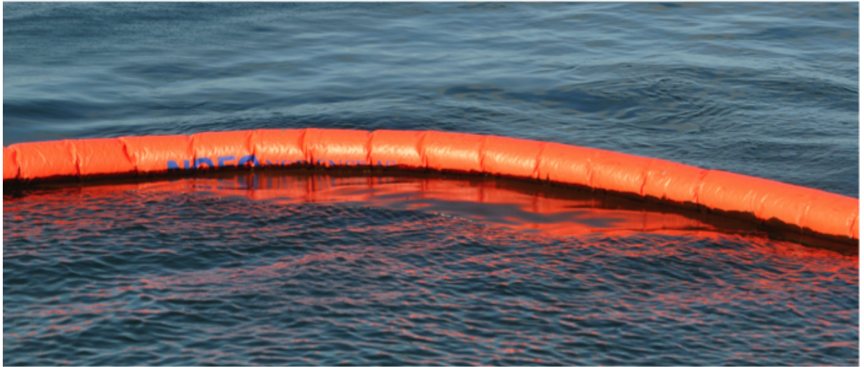
Figure 5.4: A smoother surface is seen close to the boom where the oil is collected because the oil dampens the small surface waves. Photo: Stine Skrunes.
