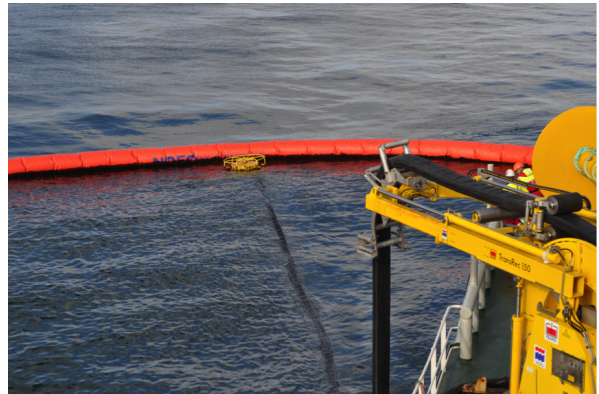
(d) Collected oil is being pumped up.
