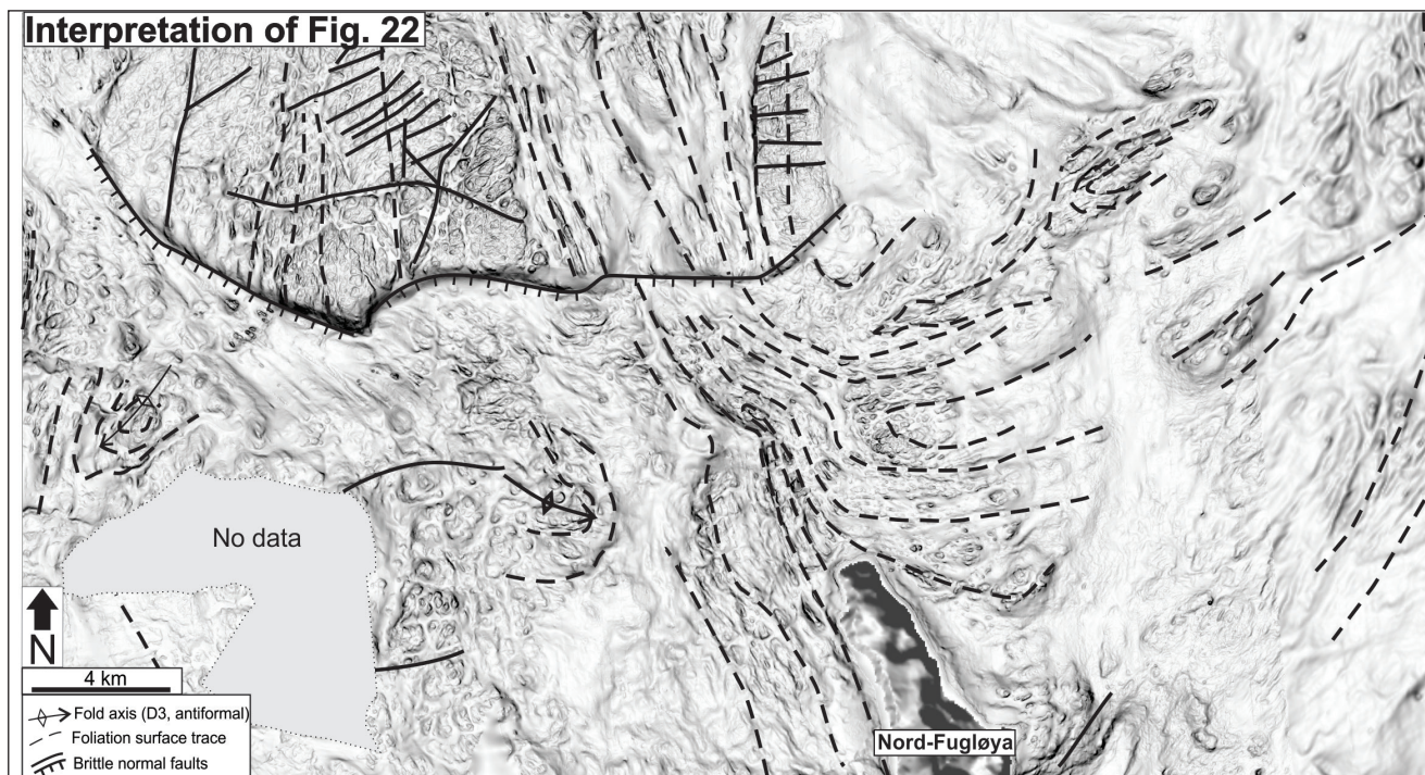
Figure 23. Detailed interpretation of the inferred WTBC – Caledonian contact and related structures covering the strandflat within Area 3 (see Fig. 21 for location), based on correlation with known onshore structures. The contact is marked by a change in the preferred orientation of NE–SW-trending ridges to the northeast, relative to NNW–SSE-trending ridges in the northwest, i.e., ridges just west of Nord–Fugløya.
