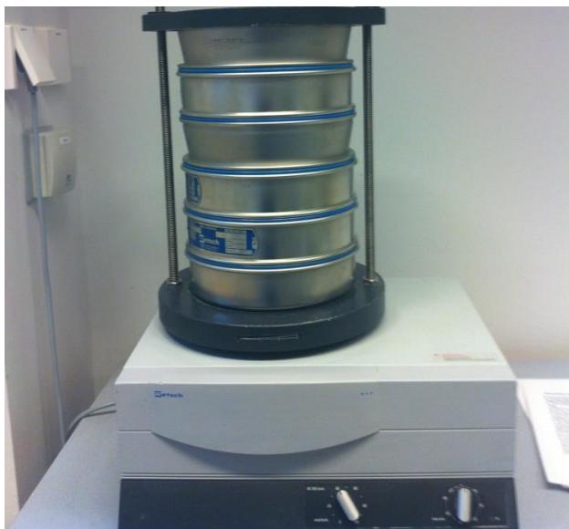
Figure 6: Retsch mechanical sieve shaker and sieves used for particle size analysis
