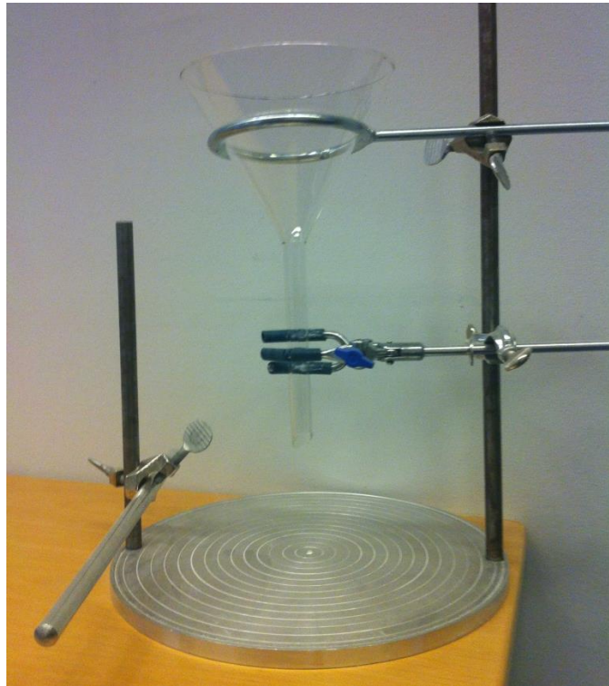
Figure 7: Showing equipment used for the test of angle of repose and flow time
