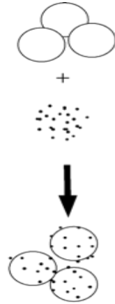
Figure 2: Illustration of interactive mixing: carrier particles coated with micronized drug particles (modified from (Bredenberg et al., 2003a))
