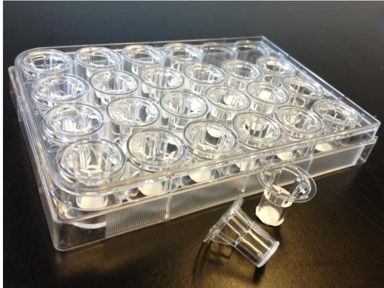
FIGURE 7: A 24-TRANSWELL PLATE WITH INSERTS
