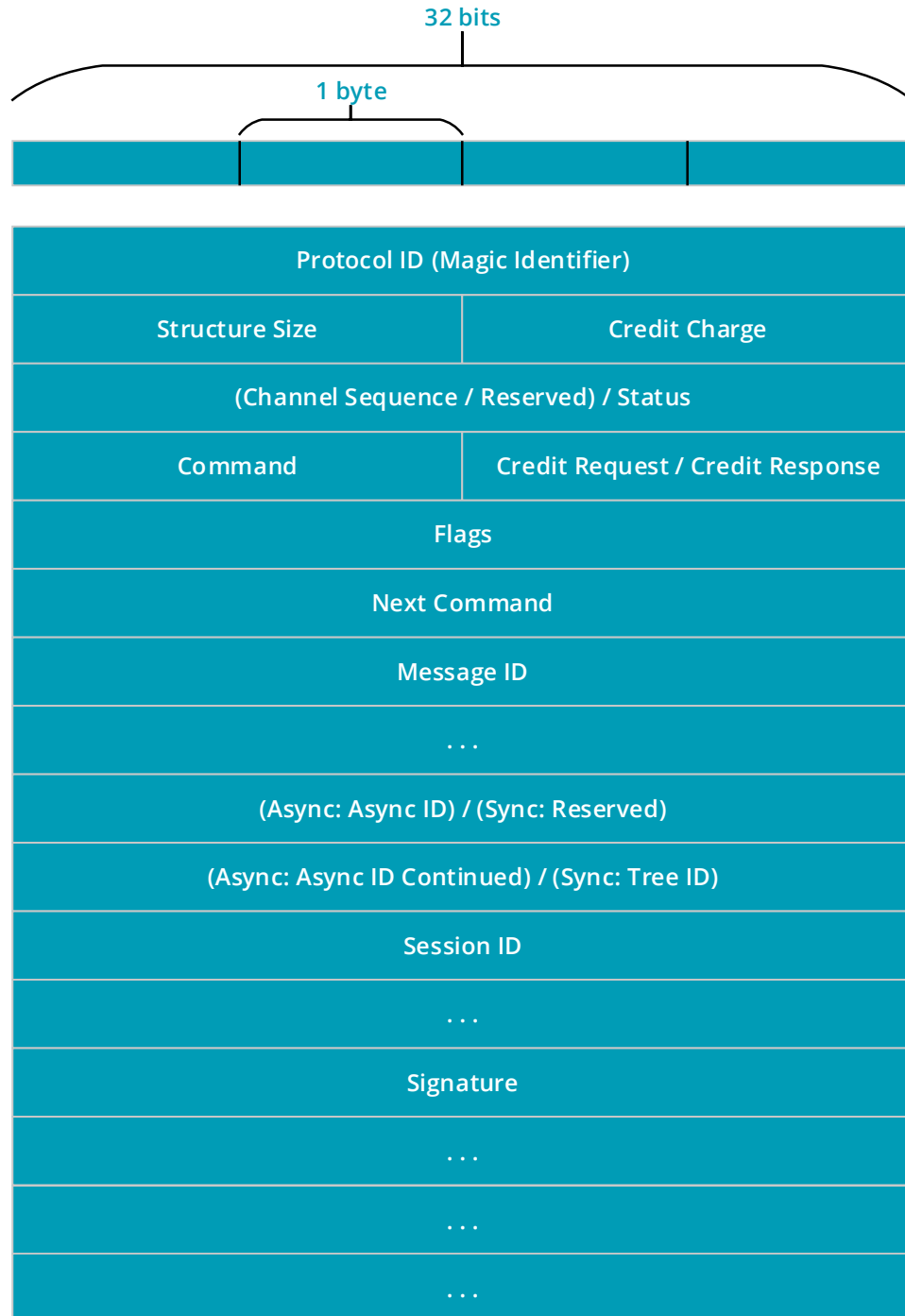
Figure 3.3: Layout of the SMB2 header.
