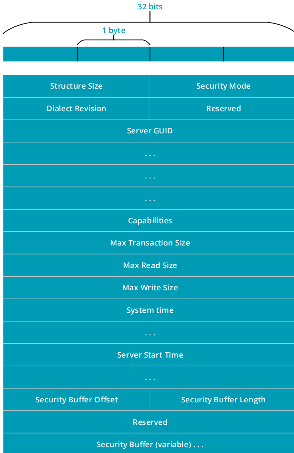
Figure 3.5: Layout of the SMB2_NEGOTIATE response command structure.
